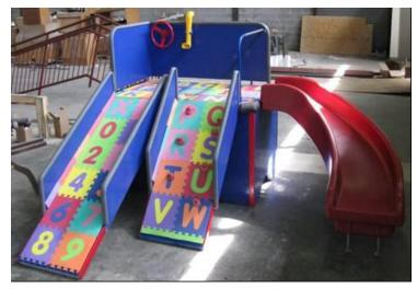
Fig. 14.7. Photo of completed climbing wall device for children at the Bell Center. The composite structure features two climbing surfaces for varying levels of ability, and the entire structure is easily disassembled for storage.
